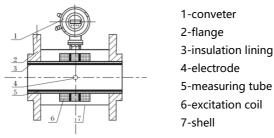
The electromagnetic flowmeter is mainly composed of two parts, the sensor and the converter. The sensors include flange, liner, motor, measuring tube, excitation coil and sensor housing. The converter comprises an internal circuit board and a converter shell.
