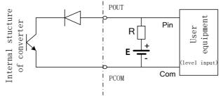
Additional remarks : pulse output for OC gate output, need external power supply. General counter all wear resistance, signal can be directly connected to the counter.
