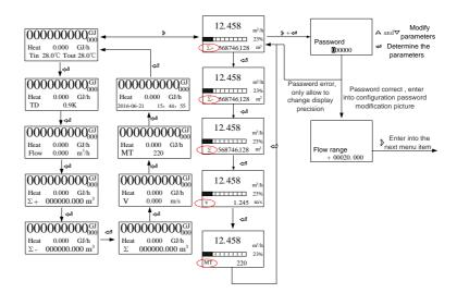
Flow setup and analog output menu
