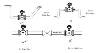
The piping design shall ensure that no gas is separated from the liquid The flowmeter should be installed upstream of the valve because the pressure in the pipe will be reduced due to the action of the valve, resulting in bubbles At the same time, instruments should be installed in the lower section to reduce the influence of entrained air bubbles on the measurement
