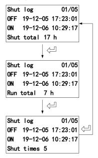
Use the  $\bigtriangleup$  and  $\bigtriangledown$  keys to switch the power-off record list on the power-down record screen.
