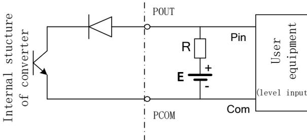
Additional remarks : pulse output for OC gate output, need external power supply.
