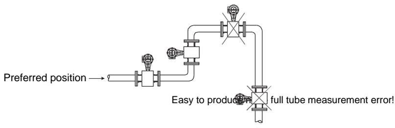
Pipe to the highest point (air bubble concentration in the measurement tube easy to generate measurement error!)
