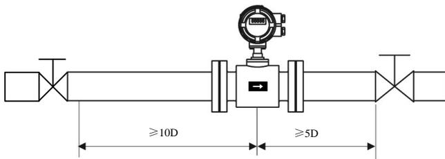
6. The two ends of the heat meter must be equipped with valves of corresponding caliber, which can be separated from the heat meter for cleaning and maintenance of the heat meter in use.
