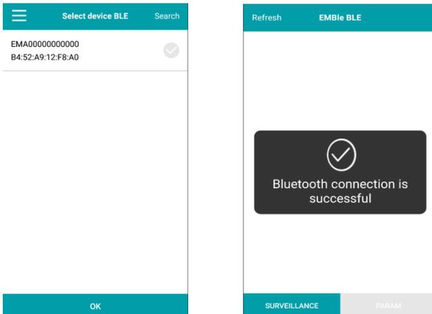
After the Bluetooth connection is successful, the parameters can be monitored and modified
