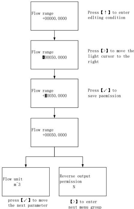
Flow setup and analog output menu
