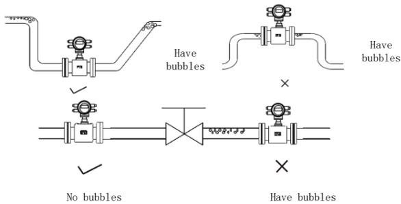
The piping design shall ensure that no gas is separated from the liquid
