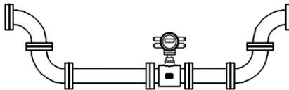
For liquid containing solid particles or the slurry suggestion vertical installation of electromagnetic flowmeter, a can prevent the phase separation of measured medium, the second lining wear can make the sensor is evener, three impurities were not able to measure the sediment at the bottom of the tube.
