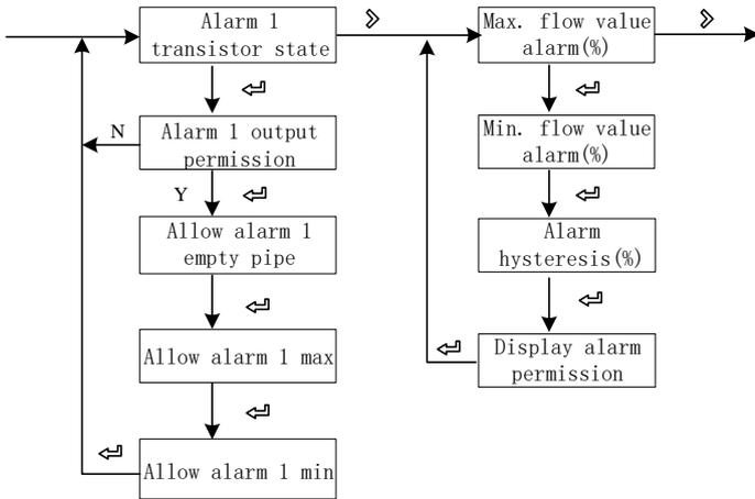
**System function, empty pipe function , sensors function, test function setup**
