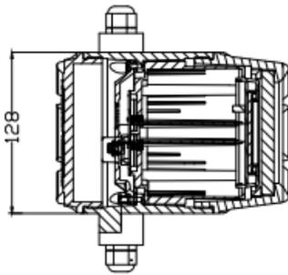
3.8 Dimensions of plug-in electromagnetic flowmeter
