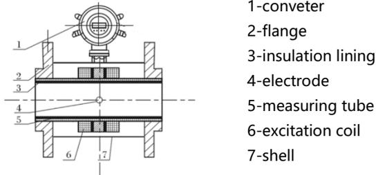
The electromagnetic flowmeter is mainly composed of two parts, the sensor and the converter. The sensors include flange, liner, motor, measuring tube, excitation coil and sensor housing. The converter comprises an internal circuit board and a converter shell.
