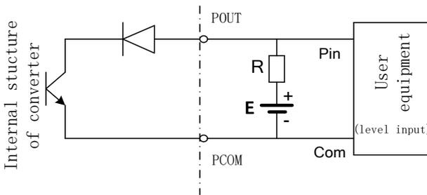
Additional remarks : pulse output for OC gate output, need external power supply. General counter all wear resistance, signal can be directly connected to the counter.
