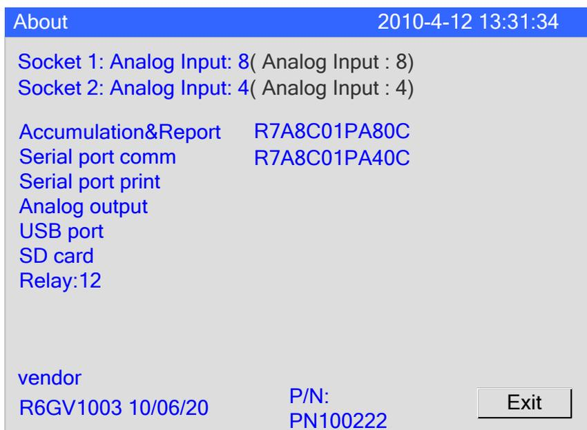
Blue Text (1: R7A8C: 8) is the inherent information in AD, black text (R7A8C: 8) is the current AD board information, if there is any difference between them, this shows that AD board failure, please contact the manufacturer for maintenance.
