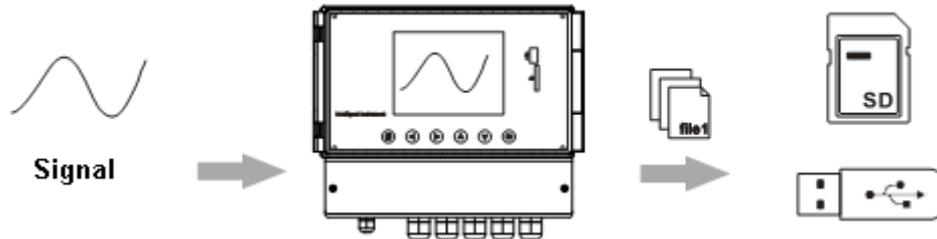
Displayed data is shown as curves and other data on meter screen. It is the data filter out from the samples by the instrument. A datum is equivalent to a point on the curve of the screen. The time of a datum is determined by recorded meter intervals. Historical data is equivalent to the original recording paper, which is very suitable for long-time observation.
