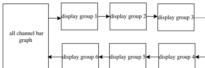
Use [Enter] to start or stop the automatic switching function of display combinations, every 5 seconds automatically switch to the next combination curve, with a status bar icons.
